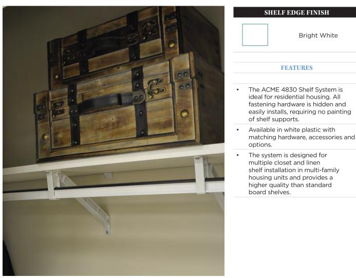
The ACME 4830 Shelf with Hanger Bar System offers a wide variety of configurations, each custom-manufactured for precise fit. A rugged vinyl cap snaps over the hanger bar sliding surface to promote easier hanger movement and excellent resistance to scratches. We recommend a center brace shelf support with hanger bar (48310) for shelving in excess of 4 ft (1.22 m) long and one for each additional 4 ft (1.22 m).
